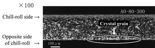
Figure 10. Optical microscope image of A0-80-300 sheet which was used to slice the surface layer of the opposite side of chill-roll. *Crystal grain depth: 26 \mu m.
